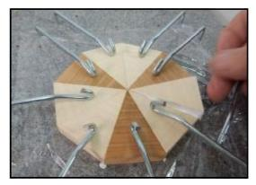
Only when you are happy with the layout do you start gluing. If you are working with an odd number of segments, remove one piece and apply glue to one edge only. Continue by
