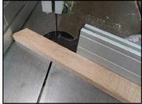
Cut one end of a piece of scrap timber, flip it over, and set the rip fence to give you the correct "max length" for your segment. You are now ready, and should proceed with cutting a set of segments.
